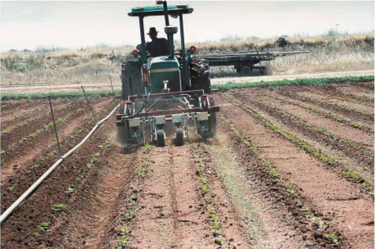
The Weedfix® cultivator is an effective implement for controlling post-emergent weeds in row crops.
