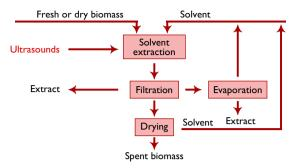
Figure 4: Sonicated-assisted extraction process diagram.
