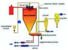
Figure 8: Spray drying process
