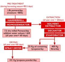
With solvent extraction it is possible to extract, during the 60 days of yearly production, around 25kg of oil containing lycopene and 400kg of fibre per day. The oil can be sold as such or further processed into lycopene powder yielding 101kg/day.
