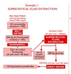
With SFE it is possible to extract, during the 60 days of yearly production, around 39kg of oil and wax containing I and 0.5% lycopene and 389kg of fibre per day. The oil and wax can be sold as such or further processed into lycopene powder (0.25%) yielding 123kg/day.
